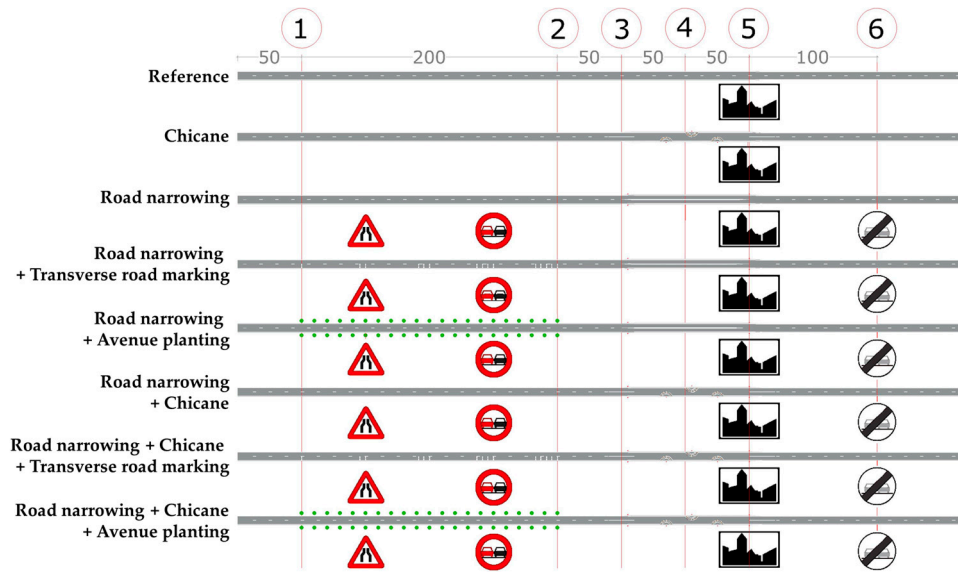
Figure 5. Measurement points for speed (distances are in meters).
